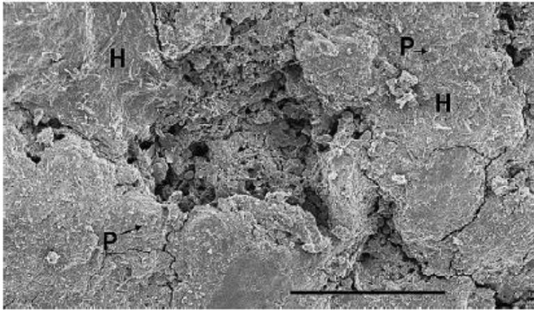
Fig. 10. SEM photo showing the circular pits (P) and fungal hyphae (H) of the patina. The sample was taken from the border between letter incision and the natural rock, near the crack zone (scale bar = 30  $\mu$ m).
